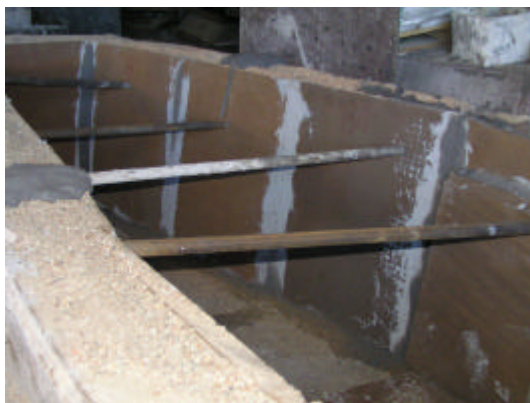
Figure 2 Insulation improvement of the tundish
