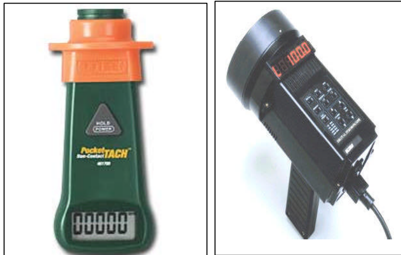
Figure 17. A tachometer (left) and a stroboscope (right) (Reliability Direct, Inc)
