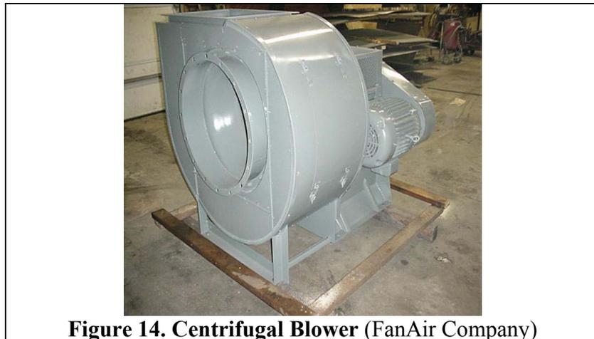
**Figure 14. Centrifugal Blower (FanAir Company)**
