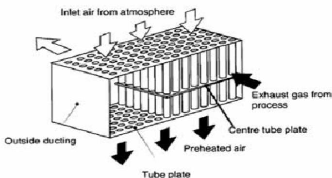
Figure 1. Waste Heat Recovery using Recuperator (SEAV, 2004)
