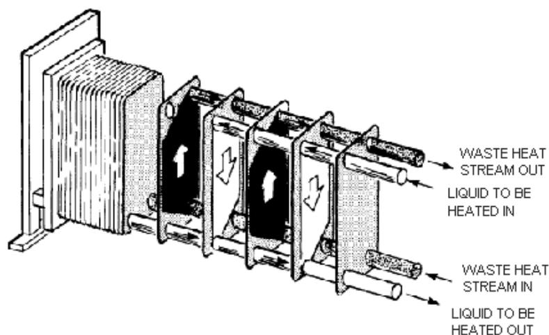
**Figure 10. Plate Heat Exchanger**
