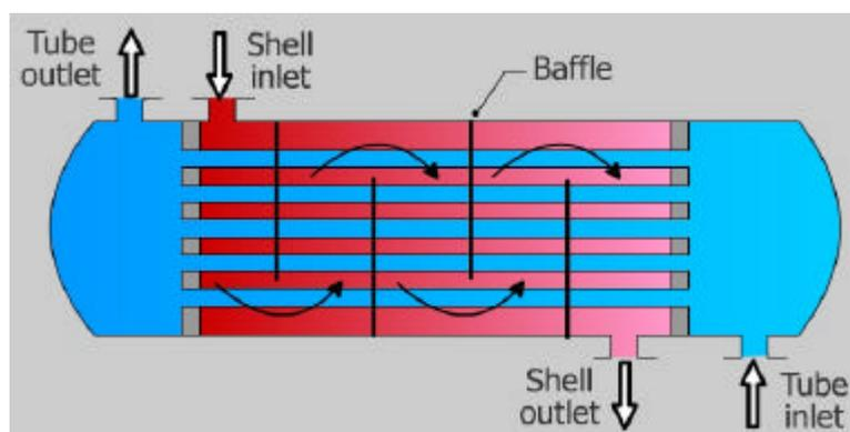
**Figure 9. Shell & Tube Heat Exchanger**
