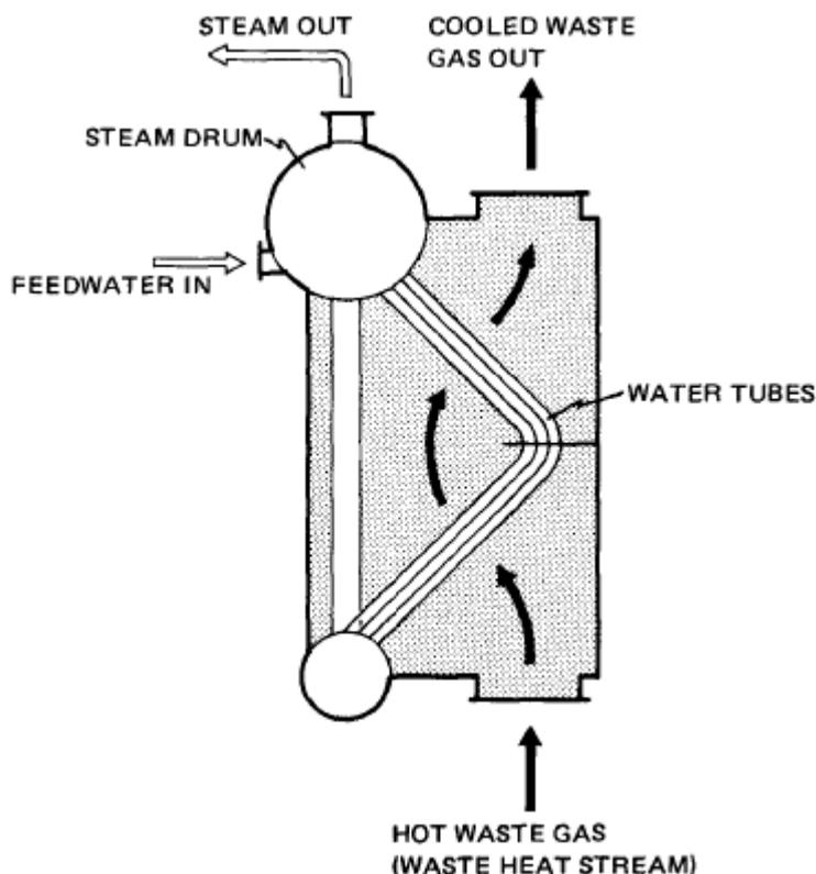
**Figure 12. Two-Pass Water Tube Waste Heat Recovery Boiler**
