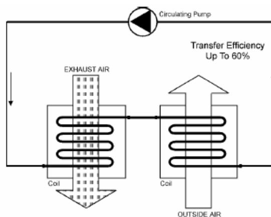
**Figure 11. Run Around Coil Exchanger**
