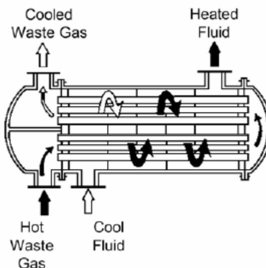
**Figure 3. Convective Recuperator** (Reay, D.A., 1996)
