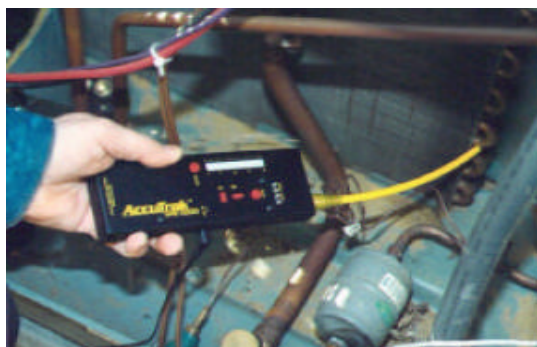
Figure 9. Ultrasonic leak detector (Tashian, Paul)
