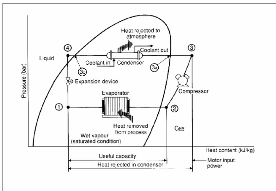
**Figure 4. Schematic representation of the refrigeration cycle including pressure changes (Bureau of Energy Efficiency, 2004)**
