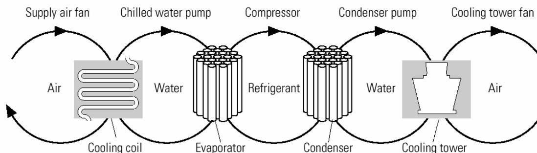
**Figure 2. A typical Heat Transfer Loop in Refrigeration System**
