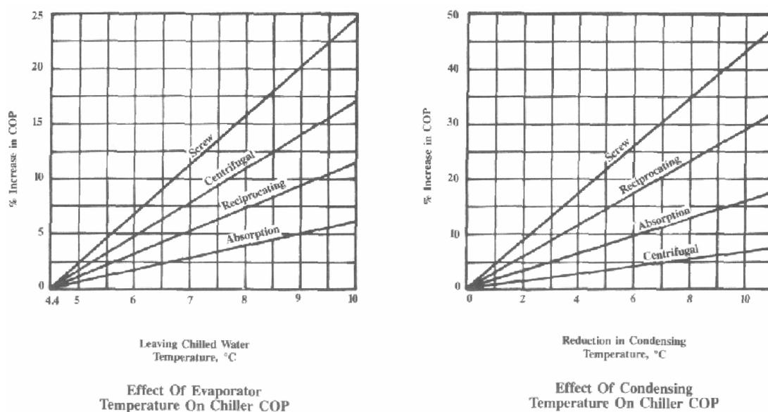
**Figure 6: The effect of condensing temperature and evaporator temperature on the chiller (Bureau of Energy Efficiency, 2004)**
