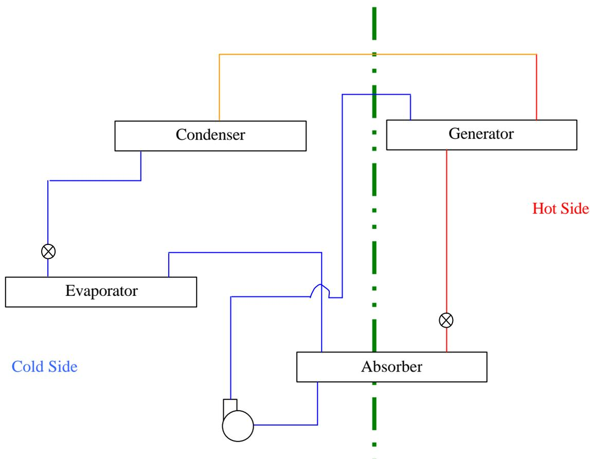
**Figure 5: A simple schematic of a vapour absorption refrigeration system**
