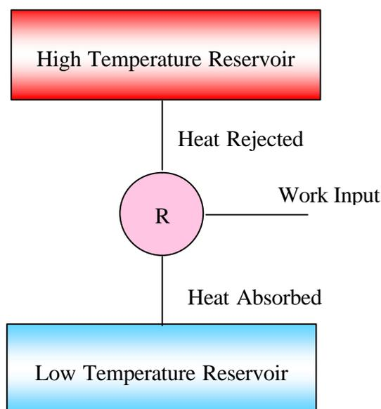
Figure 1. Schematic representation of refrigeration system
