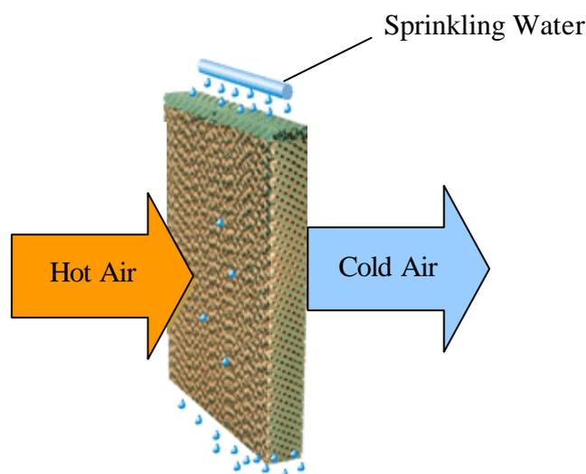
**Figure 5. Schematic of evaporative cooling**
